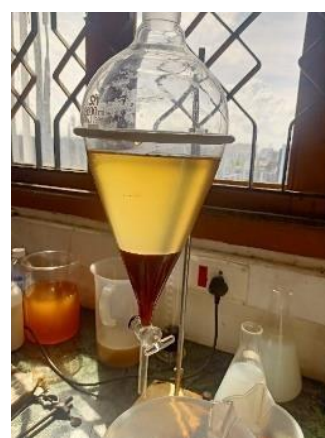
Fig. 4.2 Separation of Crude Glycerin
