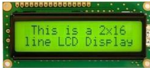
Fig 4.11: 2x16 Line Alphanumeric LCD display
