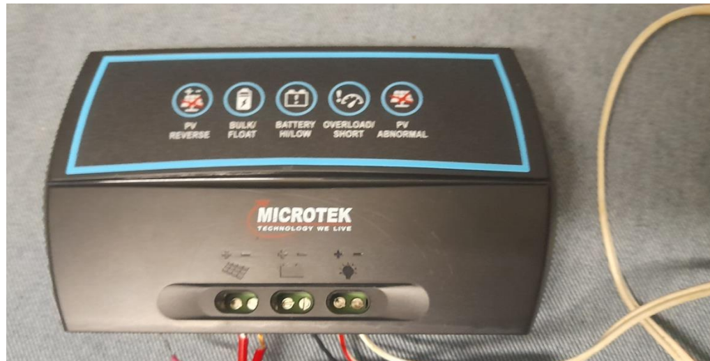
Figure 3.2.3 Picture of charge controller
