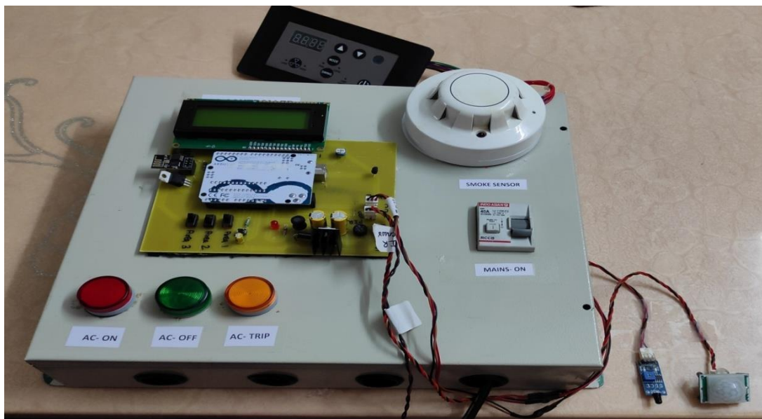
Figure 23 Prototype AC controller with IOT module
