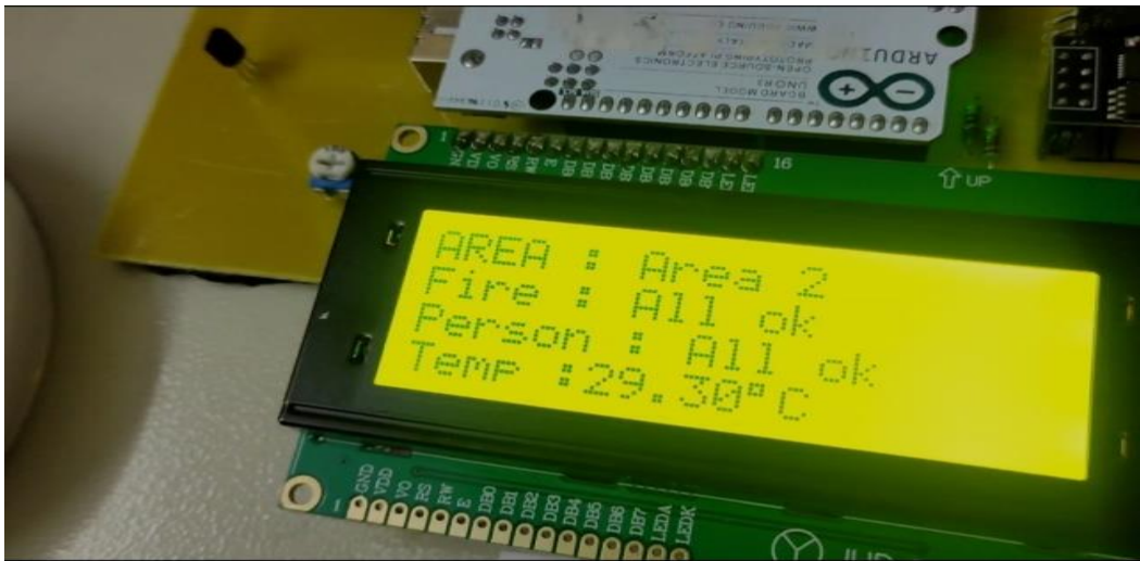
Figure 26 LCD Display showing all OK in Area- 2
