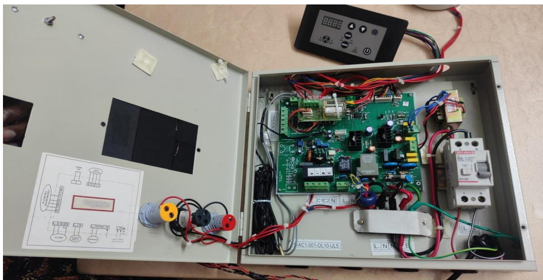
Figure 24 Inside view of AC controller
