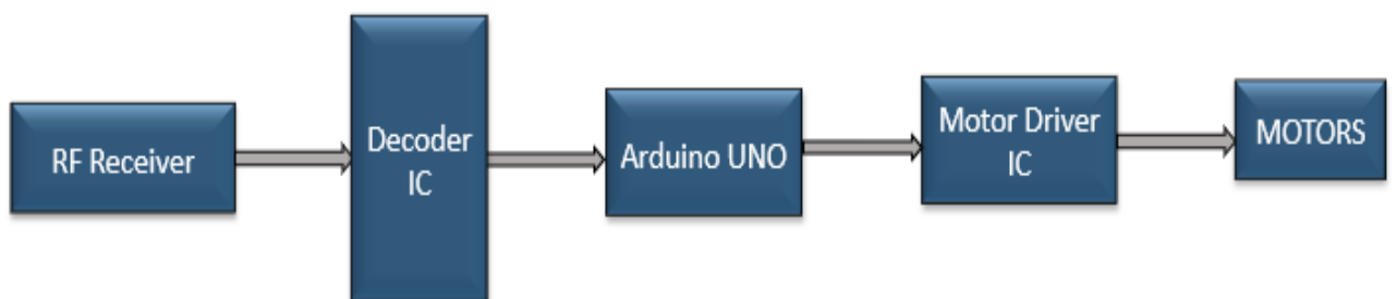
Figure 3.2: Block diagram of receiver
