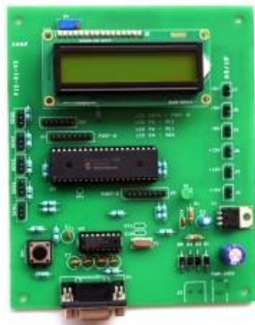
Fig. 5.5: PIC Controller Board
