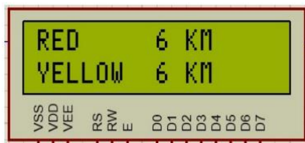
Fig:4.9 : LCD display after delay during L-L-G fault Software Simulation
