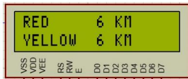
Fig:4.7 : LCD display after delay during Line to Line fault Software simulation
