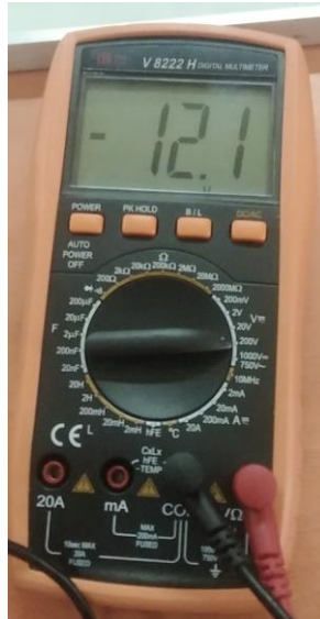
Fig 5.6 Input voltage of Landsman converter
