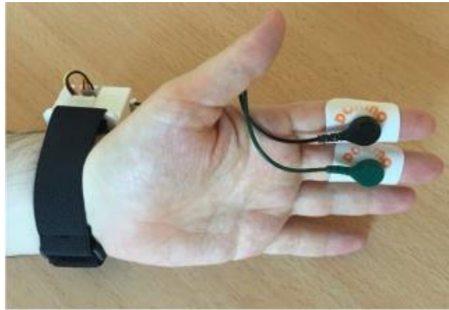
Fig 4.4 Electro dermal activity sensor (EDA)
