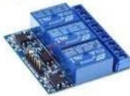
Fig 5.6 Three Channel Relay
