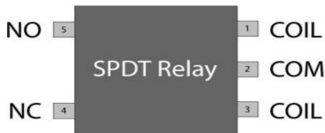
FIG 4.8: Pin diagram of Relay
