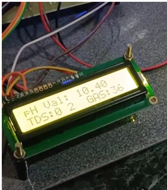
Fig 6.3: LCD display representing Alkainity of the saturated solution
