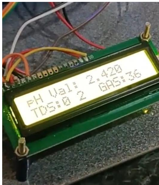
Fig 6.2 : LCD display representing acidic nature of saturated solution
