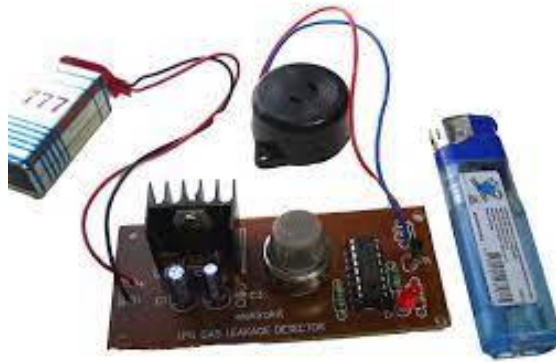
Fig 4.1: Gas leakage system and alarm system
