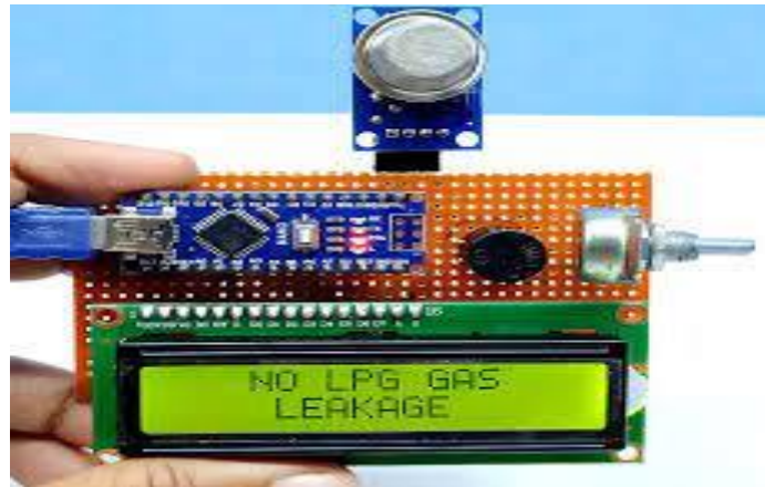
Fig 4.3: Arduino gas detection system
