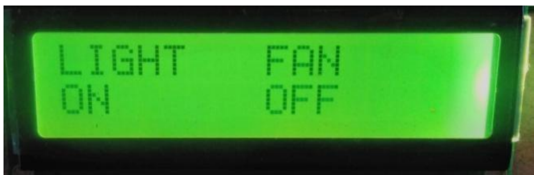
Fig.4.2..Light is in ON and Fan is in OFF condition displayed on LCD. Bluetooth technology can be used to enable speech recognition in industrial and home automation systems. Here is an overview of how it can work:
