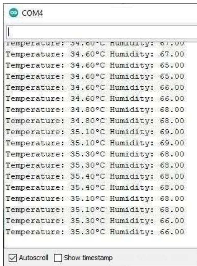
Figure 4.4.2.3 Serial Monitor Output of Humidity Temperature
