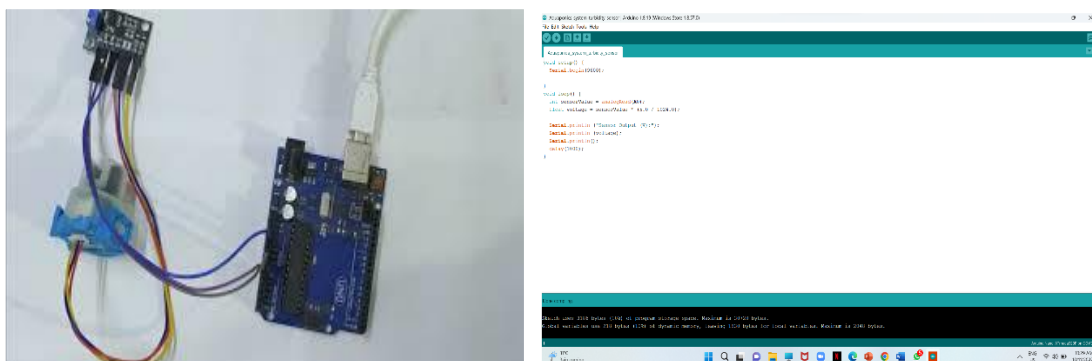
Fig: 5.3.7. Test setup for Turbidity sensor and screenshot of the code output.
