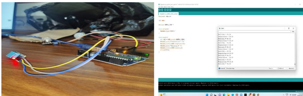
Fig: 5.3.6. Test setup for DHT11 sensor and screenshot of the code output.
