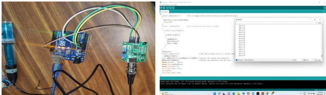
Fig: 5.3.1. Test setup for pH sensor and screenshot of the code output.
