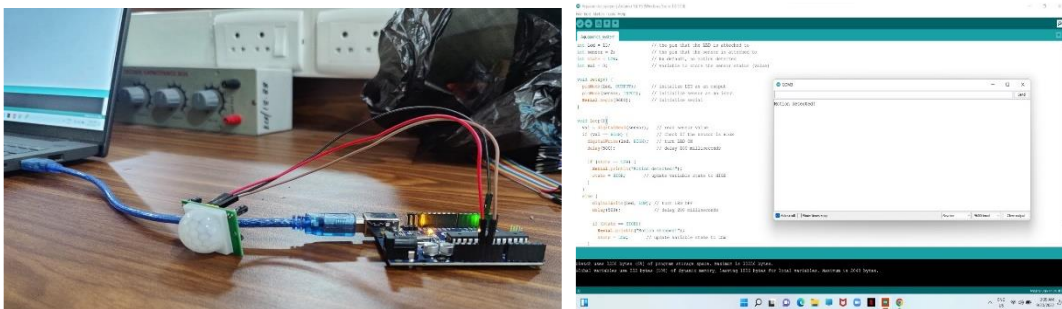
Fig: 5.3.3. Test setup for PIR sensor and screenshot of the code output.
