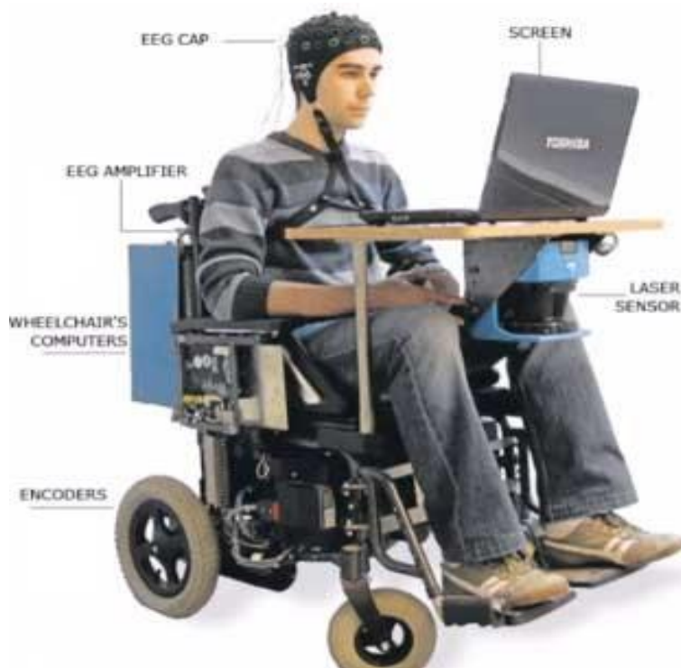
Figure 1.1 – Clip view assumption of Wheelchair with Sensor Mounts
