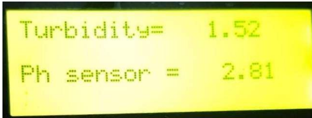
Figure.5.2.LCD displaying the water quality
