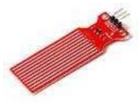
Figure.4.4. Water level sensor
