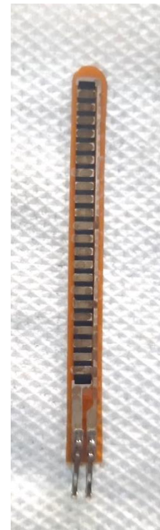
Fig 4.4: After Coating Flex Sensor
