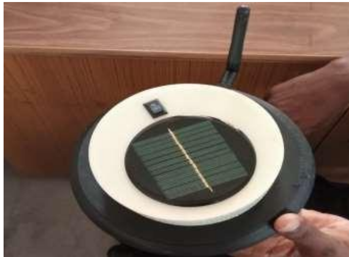
Fig 1.6: Solar panel of powering up the battery
