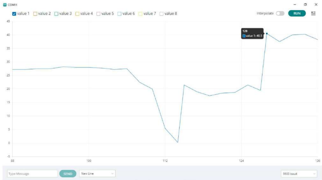
Fig 5.5 Serial Plotter output of GRID EYE SENSOR placed before HOT WATER (39-40 degrees) in graph
