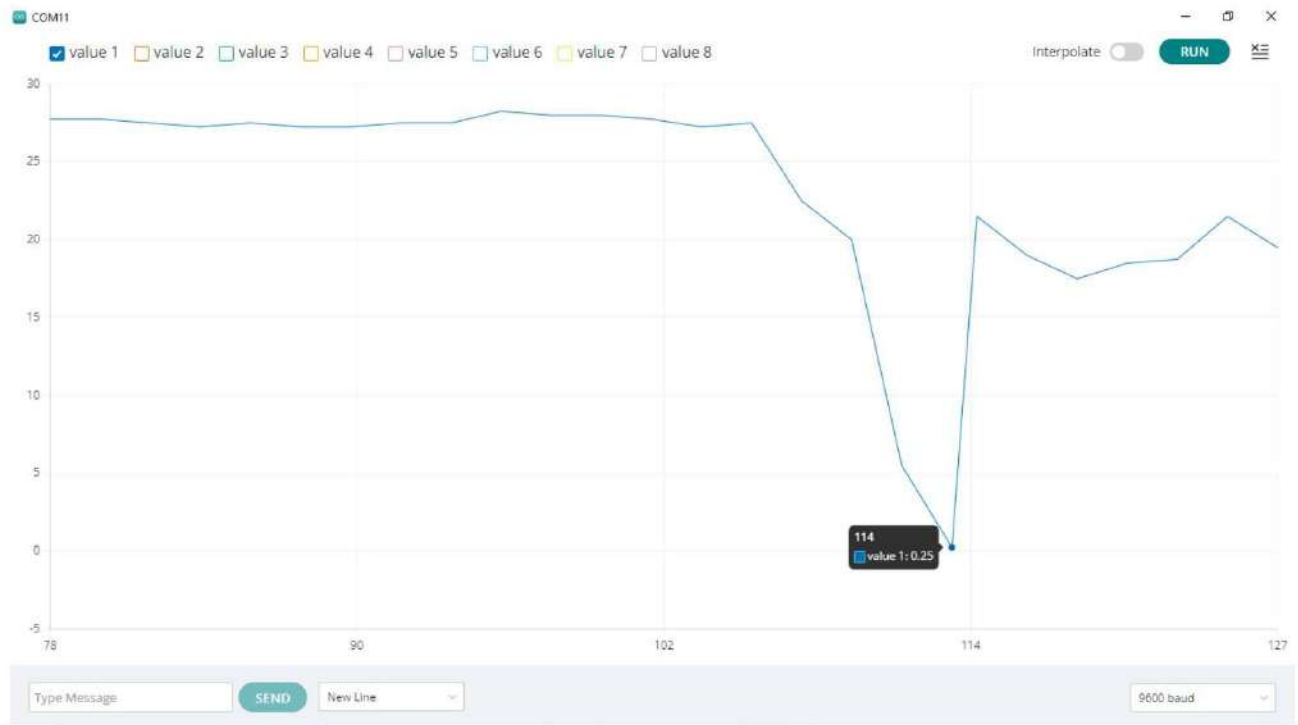
Fig 5.7 Serial Plotter output of GRID EYE SENSOR placed at COOL object (0.25 degrees) in graph
