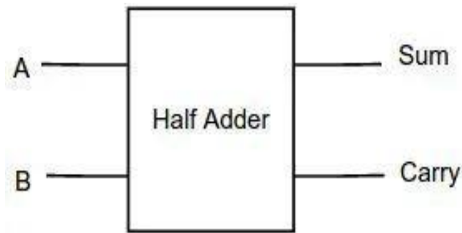
Fig 4.9 Block Diagram of Half-Adder
