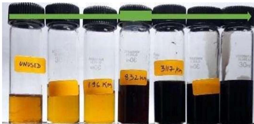
Fig.5.3. Degradation of oil sample
