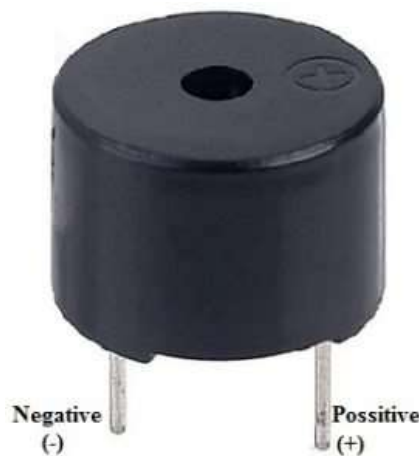
Fig 4.7. Buzzer Pin Configuration
