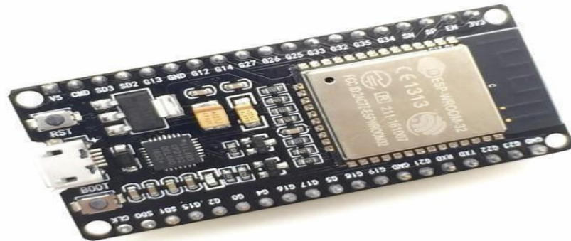
Figure 3.1 ESP32 Master Development Board
