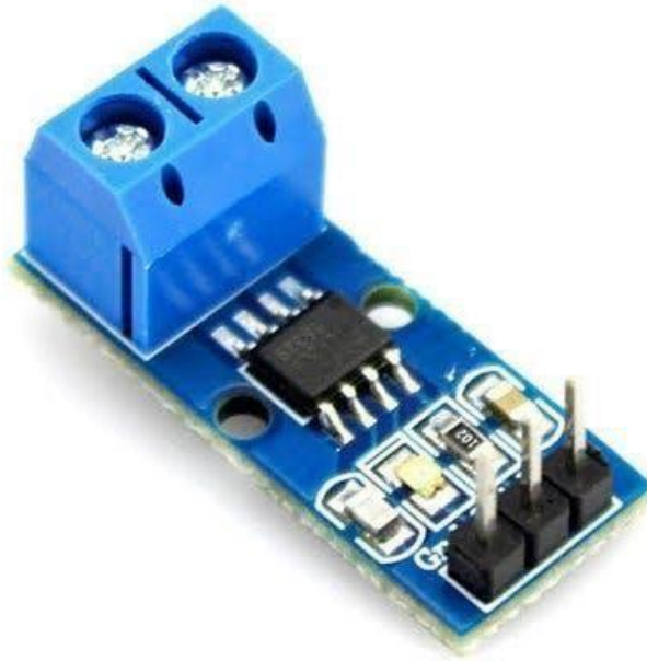
FIG 4.4 ACS712 Current Sensor
