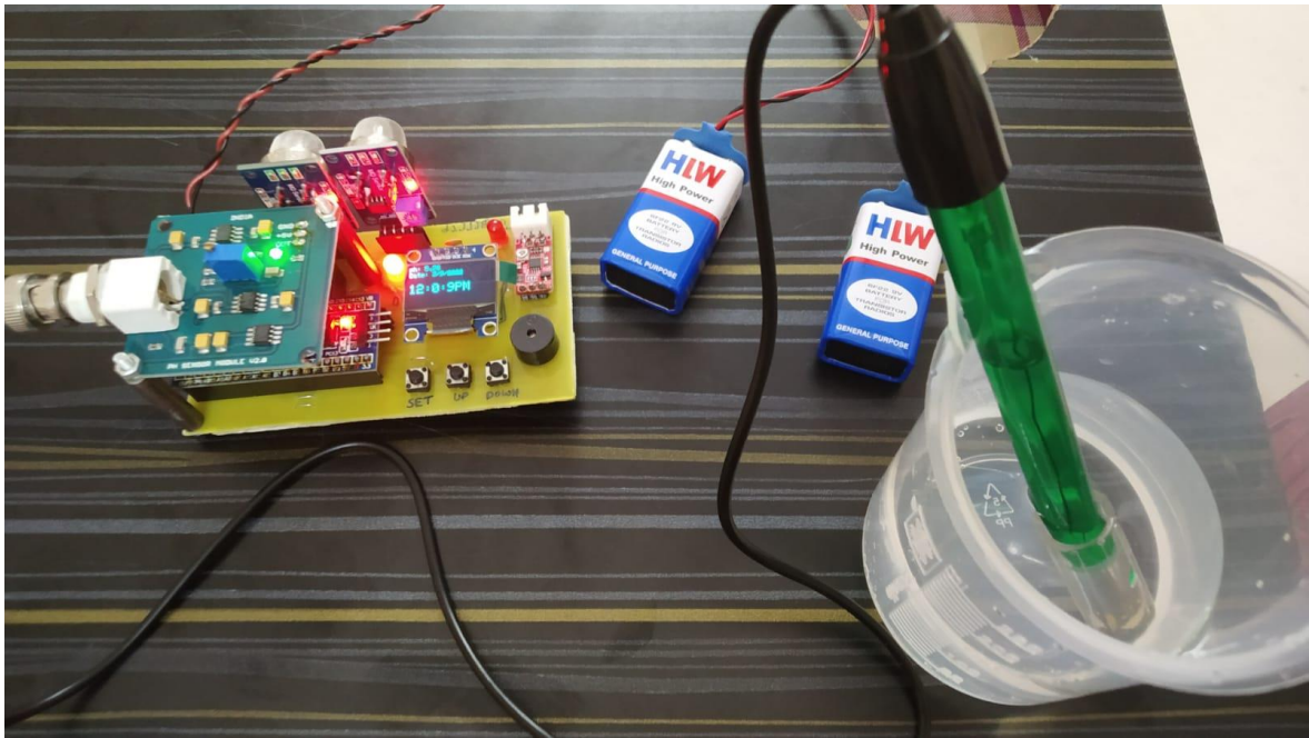
Fig 5.10 Ph of water with salt
