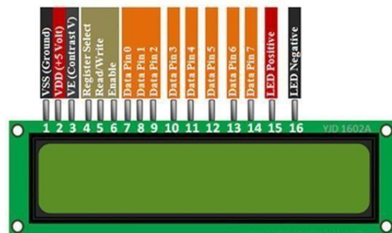
Figure 3.5.1 - 16x2 LCD (Liquid crystal display)
