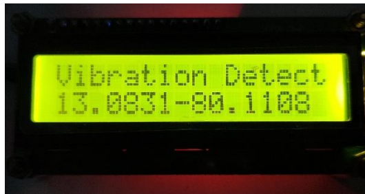
Fig.5.3: Intimating the accident coordinates on display
