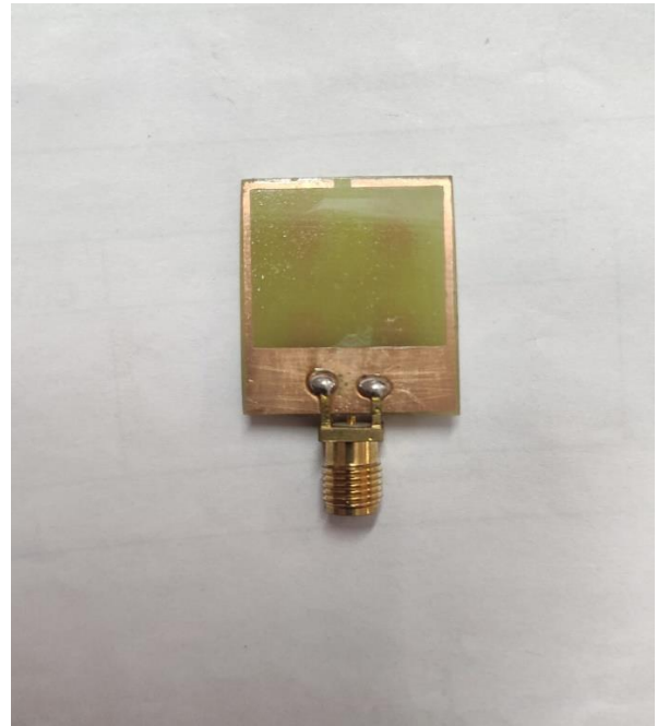
Fig 5.17 and 5.18: Front Side and Back side of the Fabricated Microstrip Patch array Antenna
