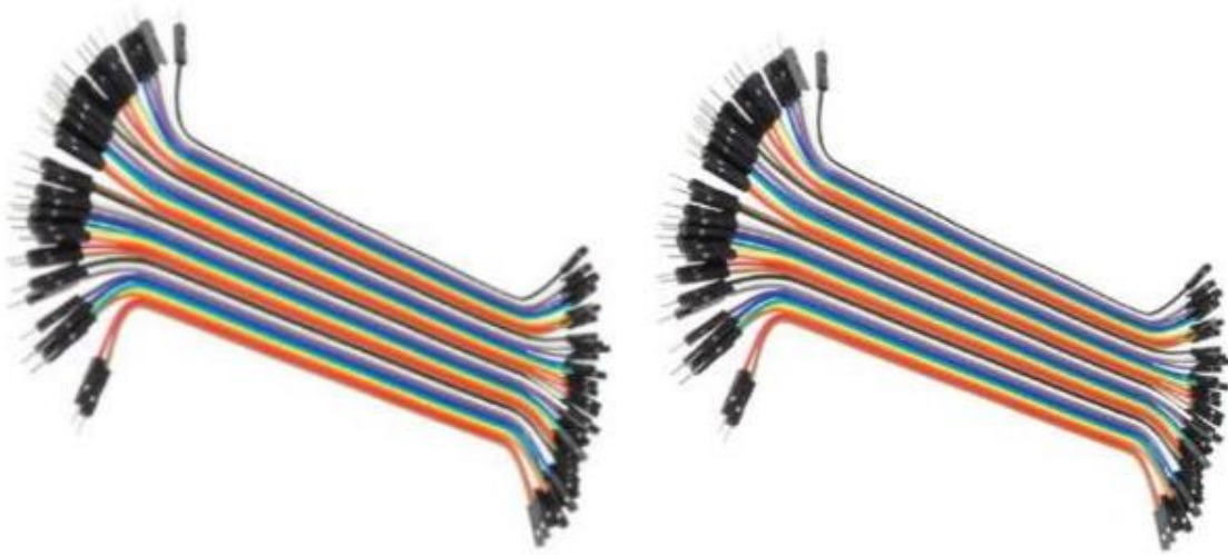
Fig 3.5 Jumper wire (M to F, M to M, F to F)
