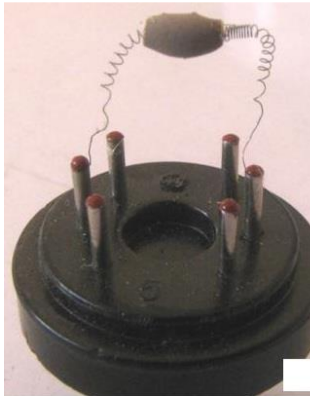
Fig 2.7 Ceramic Sensing Element Present Inside a Gas Sensor
