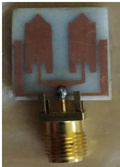
Fig 5.17: Patch design view
