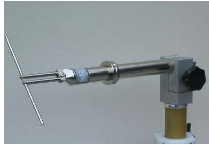
Fig:1.1: dipole antenna
