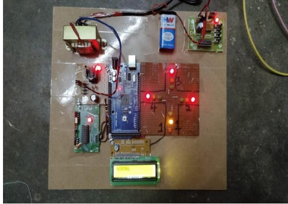
Fig 4.10 The sequence of the traffic light is going to back normal
