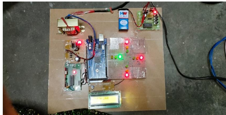
Fig 4.9 The green light of traffic light 4 is on for 10 seconds
