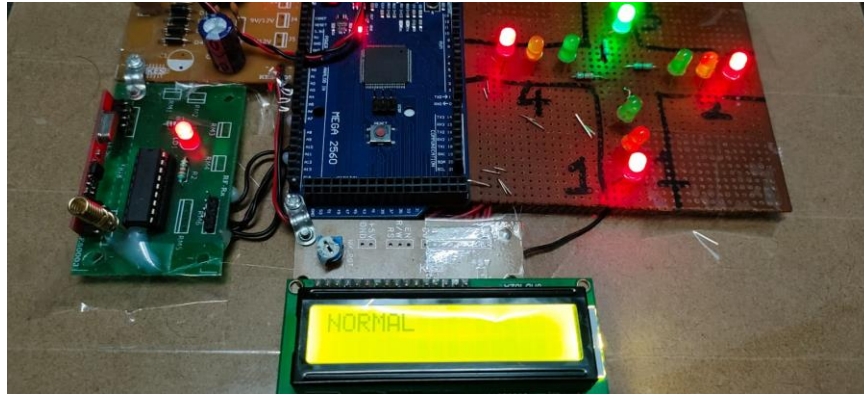
Fig 5.3 In the normal situation the green light changes from lane 2 to 3
