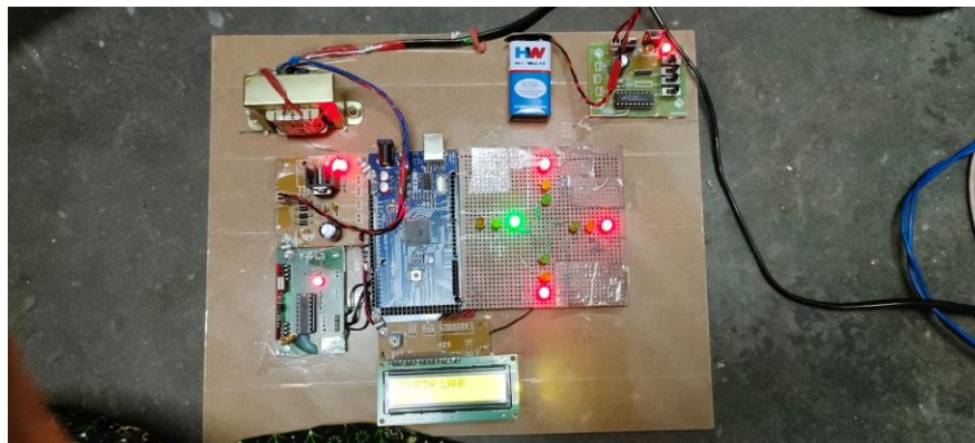
Fig 5.7 The green light is on for lane 4 for switching the fourth button
