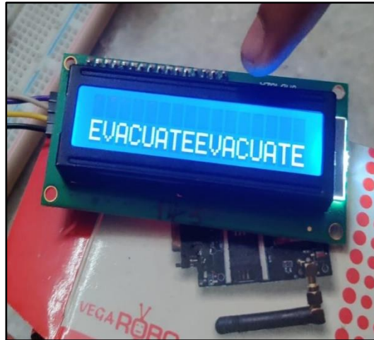
Fig.6.4 smoke detected evacuate alert message
