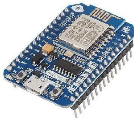
Fig :4.3 Node MCU Development Board (Version1)
