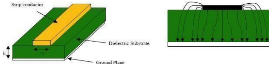
Fig. 1.3 Microstrip line and Electrical field line
