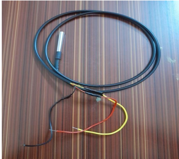
FIGURE 3.4 : TEMPERATURE SENSOR (DS18B20)
