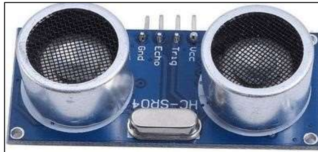
Fig.3.4 Ultrasonic sensor pin diagram
