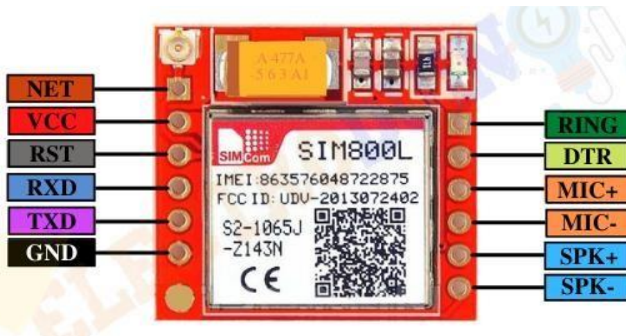
Fig 4.7: GSM Module- Pin configuration
