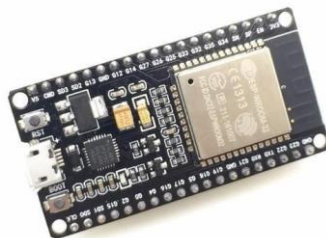
Figure 3.1 ESP32 Master Development Board
