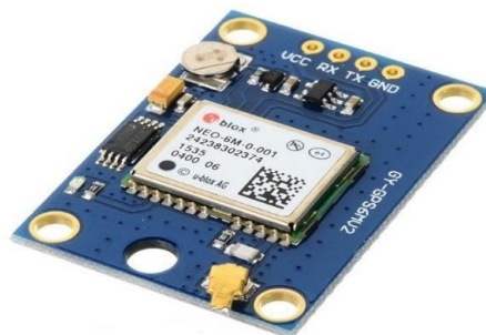
Fig. 3.2.8 GPS Pin Description
