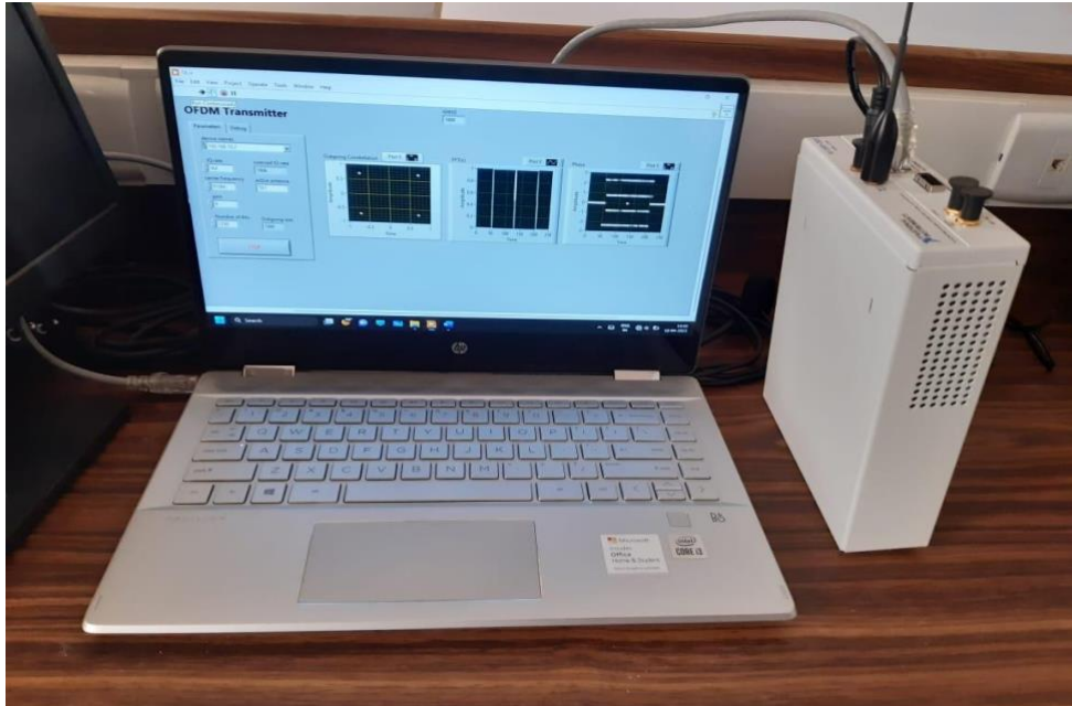
Fig 5.2 USRP real time setup for QAM Transmitter
