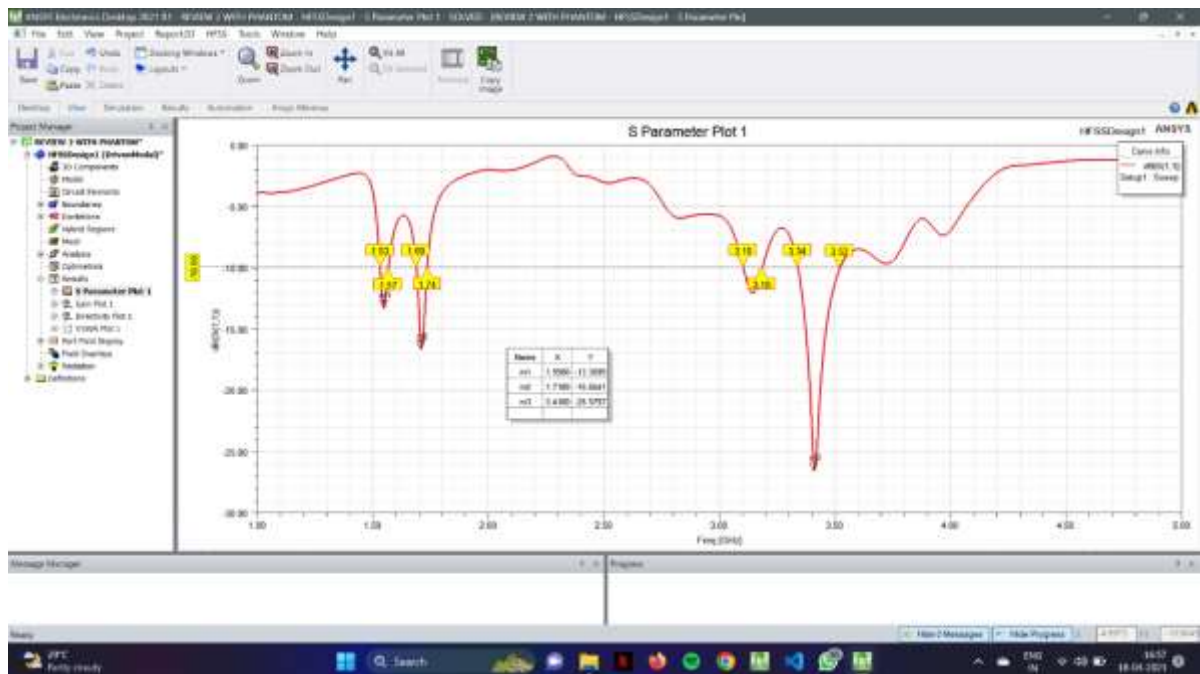
Return loss graph of UWB microstrip patch antenna design with phantom and defect
