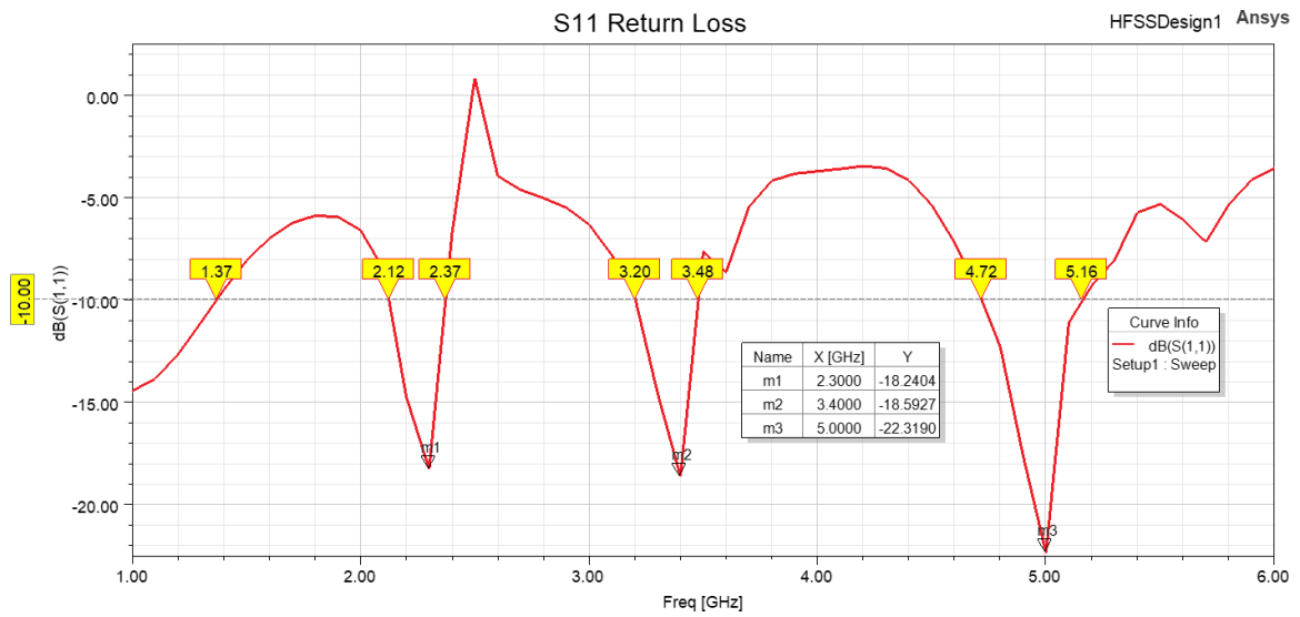
Fig 5.5 S11 Return Loss Graph
