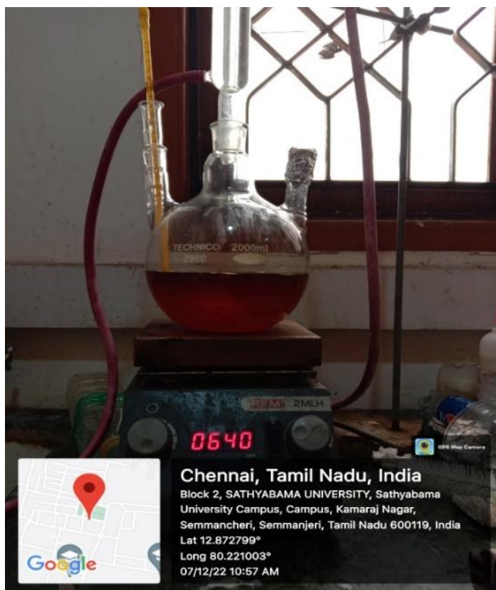
Fig 4.1. Transesterification set up
