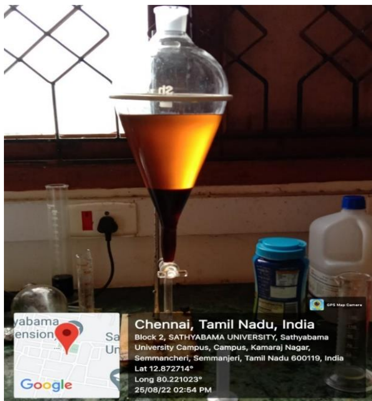
Fig 5.1. Separation of biodiesel and glycerol (Soap)
