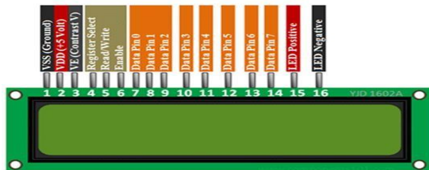
Fig : 1.6 - 16x2 LCD (Liquid crystal display)
