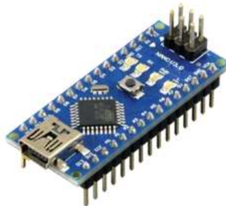
Figure 2: Arduino Nano Development module
