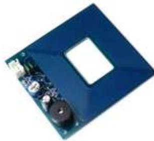
Figure 3: Metal detector module
