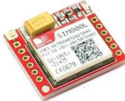
Figure 6: GSM SIM800L Module
