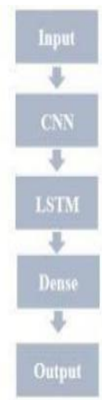
Figure 5.10 - Model Architecture of CNN-LSTM
