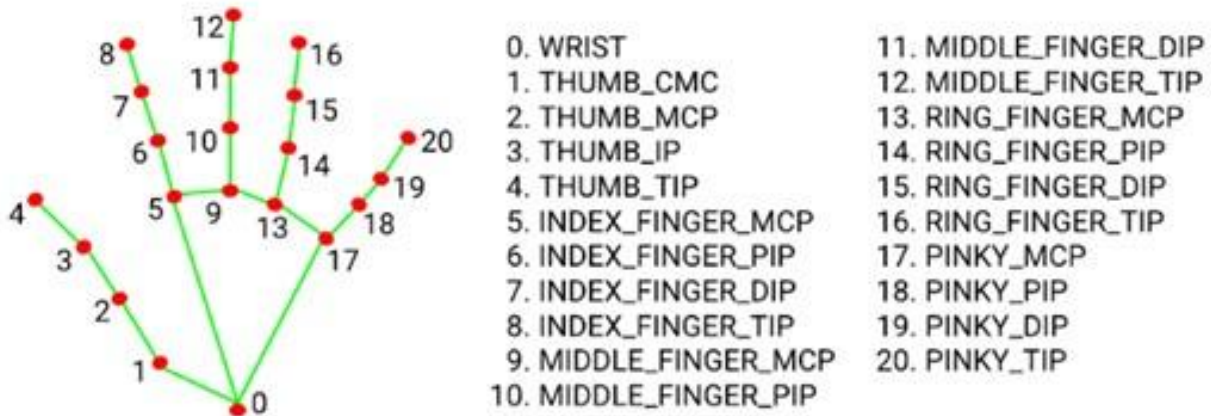
Fig. 5.2. Hand Landmarks detected by Media-Pipe
