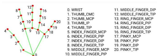
Fig. 3.2. Hand Landmarks detected by Media-Pipe, Source:[22]
